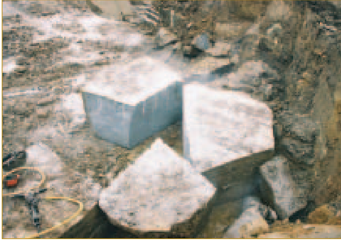
Above and right: Blockstone extraction at Appleton Quarry, using traditional 'plug & feather' techniques to split the stone and mechanical excavators to lift the blocks:
